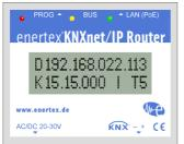
LCD shows product name and firmware version at startup. Boottime is about 2 seconds.
