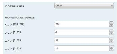
**Routing Multicast Address** This address will be used for routing telegrams on IP side. The Multicast IP Address 224.0.23.12 has been reserved for this purpose (KNXnet/IP Routing). If you want to assign another address it has to be in the range between 224.0.0.0 and 239.255.255.
