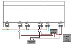
At maximum three power supplies can be connected in parallel.
